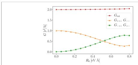
**Figure 5.** Total conductance  $G_{\text{tot}}$  and polarised spin conductances  $G_{ij}$  with  $i, j = \pm$  as a function of  $R_0$ . The systems is a slab of Na<sub>3</sub>Bi with dimensions 150 × 150 × 100 Å<sup>3</sup> and  $L_{\text{RSOC}} = 50$  Å.
