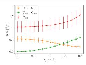
**Figure 8.** Average conductance in the presence of point-like impurities of strength  $W_0 = 0.5$  eV and density  $n_{\rm imp} = 4 \times 10^{19} \ {\rm cm}^{-3}$ . The rest of parameter are the same of figure 5. Results are averaged over 250 realizations of disorder and error bars correspond to the standard deviation.
