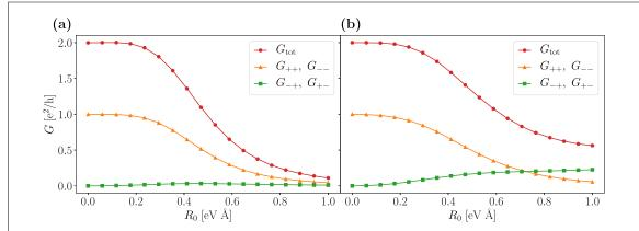
**Figure 7.** Total conductance  $G_{\text{tot}}$  and polarised spin conductance  $G_{ij}$   $(i, j = \pm)$  as a function of the RSOC coupling constant  $R_0$ . (a) Slab of DSM with the same parameters as Na<sub>3</sub>Bi but setting the quadratic terms to zero, i.e. with  $c_0 = c_1 = c_2 = 0$ . The dimensions are  $150 \times 150 \times 100 \text{ Å}^3$ . (b) Na<sub>3</sub>Bi sample of size  $80 \times 150 \times 40 \text{ Å}$  and  $L_{\text{RSOC}} = 50 \text{ Å}$ .
