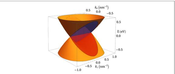
**Figure 1.** Dispersion relation for  $k_y = 0$ . Bulk states (see equation (3)) are plotted in orange, surface states (see equation (8)) in opaque red and light-blue for  $\zeta = -1$  and  $\zeta = 1$ , respectively. The parameters are  $m_0 = 0.35$  eV,  $m_1 = 1.0$  eV nm<sup>2</sup>, and v = 1.0 eV nm.
