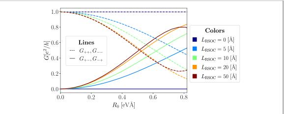
**Figure 6.** Polarized spin conductance  $G_{\pm\pm}$  (in dashed line) and  $G_{\pm\mp}$  (in solid line) for a range of  $L_{\rm RSOC}$  highlighted with the colors defined in the legend. The legend  $L_{\rm RSOC}=0$  Å corresponds to the case with no Rashba coupling.
