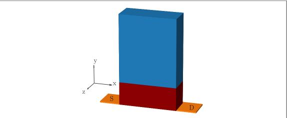
**Figure 3.** Schematic view of the device. The metallic leads are represented in orange with S and D indicating the source and the drain, respectively. The red color marks the part where the RSOC is considered whereas the blue part indicates the pure DSM without coupling.
