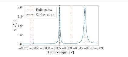
**Figure 4.** Conductance as a function of the Fermi energy; the sample in the case of  $Na_3Bi$  for  $R_0=0$  and a slab of size  $100\times250\times40$  Å<sup>3</sup>. The eigenvalues of the system are marked with black (red) vertical lines for surface (bulk) states.
