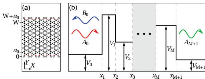
FIG. 2. (Color online) (a) Scheme of a GNR of width  $W = 8a_0$ . The boundary conditions for wave functions can be obtained by adding two rows of atoms (plotted in gray) at  $y = 0$  and  $W + a_0$  and setting the wave function to 0 in those points. (b) Transmission across a series of  $M$  potential steps. The incident plane wave with amplitude  $A_0$  splits into a reflected and a transmitted component with amplitudes  $B_0$  and  $A_{M+1}$ , respectively.
