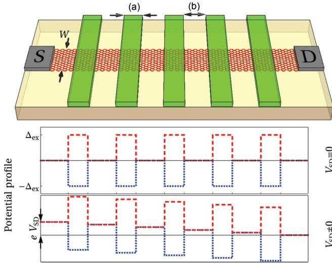
FIG. 1. (Color online) The upper panel shows the GNR connected to source (S) and drain (D) leads, with  $N = 5$  perpendicular strips of a ferromagnetic insulator (green bars) on top of it. The model potential profiles for spin-up (dashed red lines) and spin-down (dotted blue lines) electrons in the unbiased and biased device are shown in the middle and lower panels, respectively.
