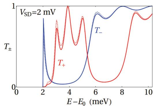
FIG. 5. (Color online) Transmissions  $T_{\pm}$  for both spins at finite bias  $V_{SD} = 2$  mV, assuming that the voltage drop occurs at the edges of the EuO strips (solid) or linearly along the sample (dashed). Here, we use the tight-binding model, which can be compared with the Dirac approximation on Fig. 4(b).
