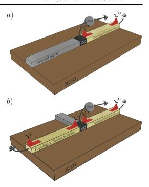
conductance in a TS-QD-N (here, TS stands for topological superconductor) and a T-shape structure with a QD connected to two topological superconductors and a normal metal).
