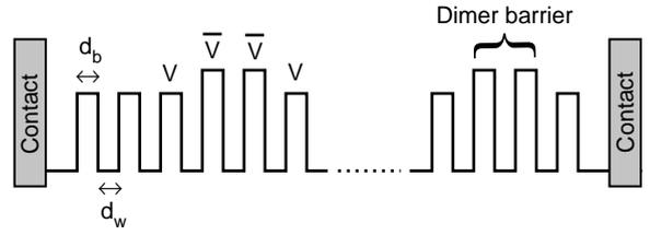
Fig. 1. Schematic view of the conduction band-edge profile of the DBSL, where pairs of  $\bar{V}$  barriers appear at random.
