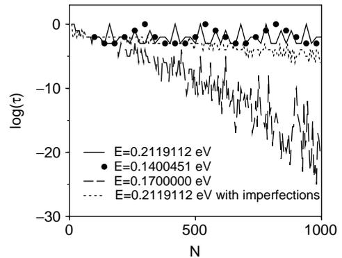
Fig. 3. Dependence of the transmission coefficient on the system size (number of periods  $N$ ). (—) and (●) correspond to  $E_c$  and  $E_d$ , respectively, whereas (---) corresponds to  $E = 0.170 \text{ eV}$ . The (· · · · ·) corresponds to the unintentionally disordered SL at  $E_c$ , where the widths of barriers and wells fluctuate 1% around their mean values.
