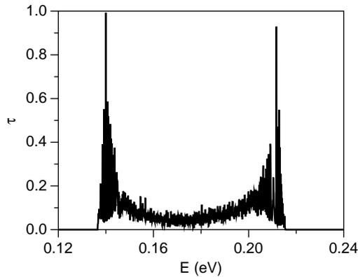
Fig. 2. Transmission coefficient as a function of energy for a DBSL with  $d_b = 25 \text{ \AA}$ ,  $d_w = 25 \text{ \AA}$ ,  $x = 0.3$ ,  $\bar{x} = 0.44$  and  $N = 1000$  periods. The fraction of dimer barriers is 30%. Two resonances can be seen at  $E = E_d \simeq 0.140 \text{ eV}$  and  $E = E_c \simeq 0.212 \text{ eV}$ .
