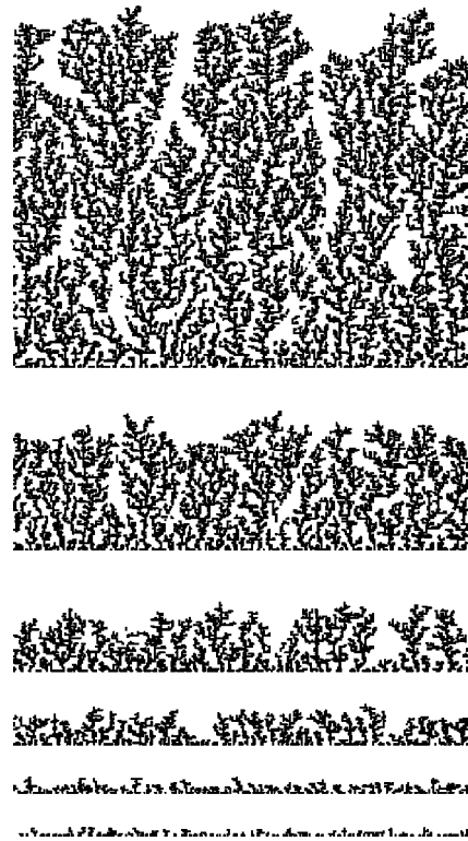
FIG. 10. Sequence of snapshots of the evolution of an aggregate grown with MBDLA without SD. Parameters are p=0.75 , s=1 , r=1 (i.e., no surface diffusion). Times (in our units, see text) are (top to bottom) 35 \times 10^6 , 17.5 \times 10^6 , 8.75 \times 10^6 , 5.25 \times 10^6 , 3.5 \times 10^6 , and 1.75 \times 10^6 .
