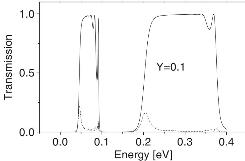
**Figure 5.** Effect of Al fluctuations in Gaussian SLs. Solid curve, average transmission. Dashed curve, standard deviation. Calculations performed with the disorder parameter  $Y$  as specified in the figure.
