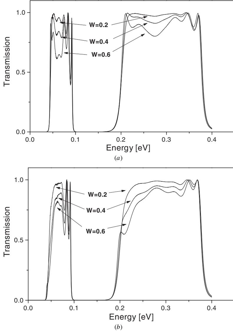
**Figure 3.** Transmission coefficient in two specific cases, (a) and (b), of vertical disorder. In each of the two figures we kept the same sequence  $\{\varepsilon_n\}$  and varied the disorder parameter  $W$ .
