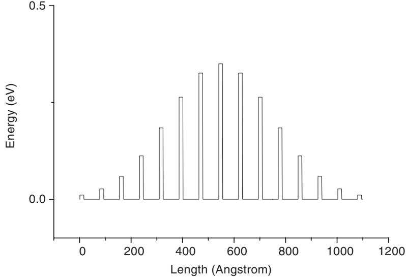
**Figure 1.** Profile of the conduction band energy of the Gaussian SL. The parameters used are as in the calculation.
