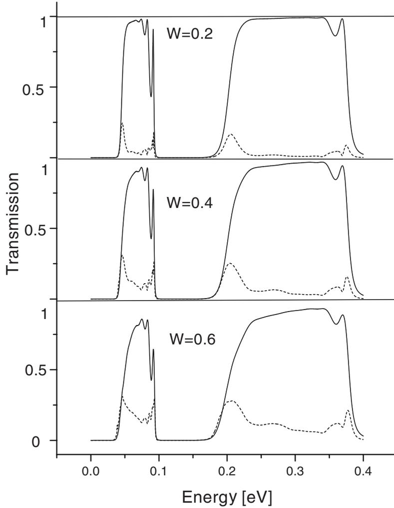
**Figure 2.** Effect of vertical disorder in Gaussian SLs. Solid curve, average transmission. Dashed curve, standard deviation. Calculations are performed with the disorder parameter  $W$  as specified in the figure.
