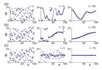
FIG. 2. (Color online) Snapshots of spatial phase profiles. (a)  $\lambda/\kappa = 0$ , (b)  $\lambda/\kappa = 10$ , and (c)  $\lambda/\kappa = 10^4$ . Each dot represents an oscillator. In all panels,  $\kappa = 1$ , r = 1, and N = 100.
