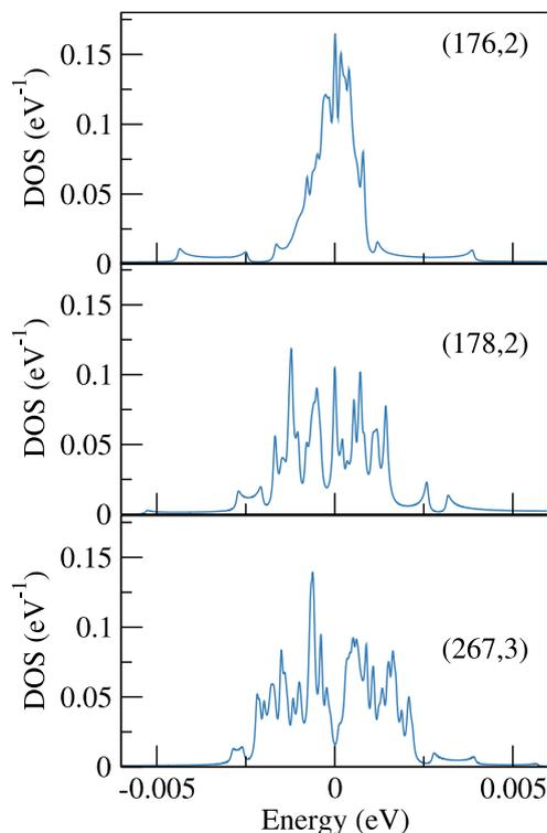
Fig. 8. From top to bottom: DOS around the Fermi energy of the 2/3-metal nanotube (176, 2) ( $\theta_M = 1.12^\circ$ ), the semiconductor nanotube (178, 2) ( $\theta_M = 1.11^\circ$ ) and the  $\Gamma$ -metal nanotube (267,3) ( $\theta_M = 1.11^\circ$ ).
