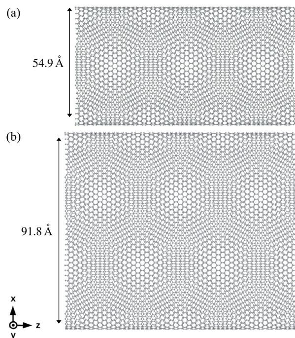
Fig. 1. Top view of the unit cells of the (a) collapsed semiconducting (48,2) and (b)  $\Gamma$ -metal (78,3) nanotubes. The number and placement of the AA regions differ and depend on the symmetry operations of the original cylindrical tube.
