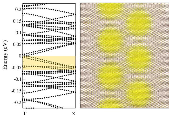
Fig. 6. Band structure and top view of the (132,3)  $\Gamma$ -metal nanotube. The LDOS of the marked bands is highlighted in yellow. (For interpretation of the references to color in this figure legend, the reader is referred to the web version of this article.)
