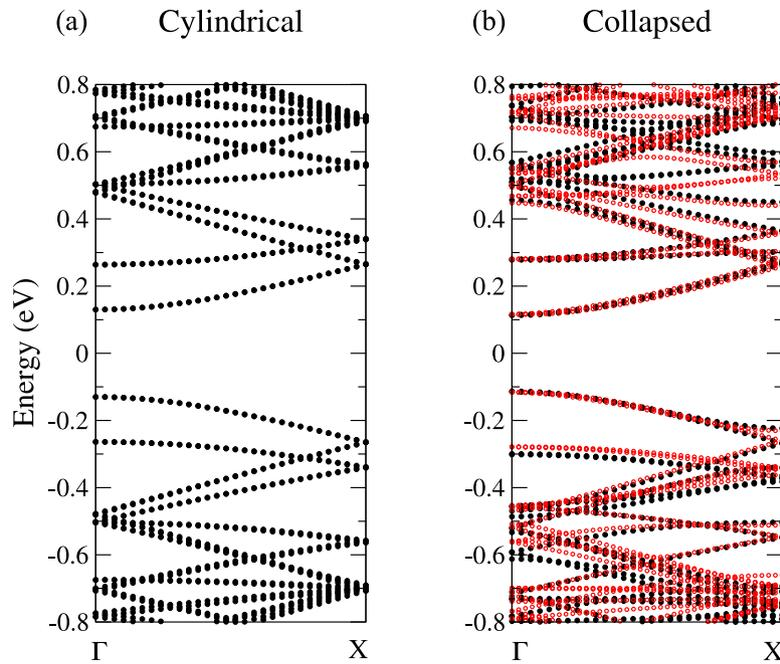
Fig. 2. Band structures of the (36,2) CNT with  $\theta_M = 5.36^\circ$ : (a) for the cylindrical geometry, obtained with the tight-binding model; (b) for the collapsed structure, obtained with both tight-binding (black) and DFT (red) calculations. (For interpretation of the references to color in this figure legend, the reader is referred to the web version of this article.)
