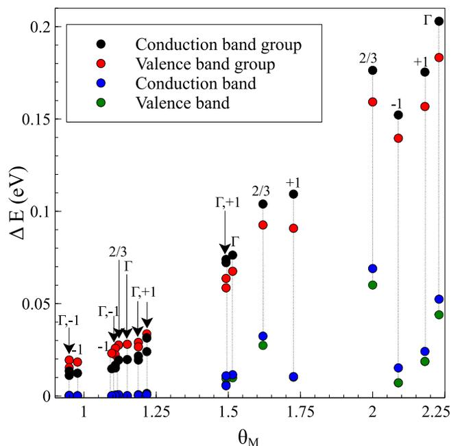
Fig. 7. Energy spans for the sets of flat bands in all kinds of CNTs. 2/3 and  $\Gamma$ -metals are labeled 2/3 and  $\Gamma$ , respectively, whereas the two subfamilies of semiconductors are labeled  $\pm 1$ . The energy widths of the pair of innermost bands, denoted by conduction and valence bands, is also shown.
